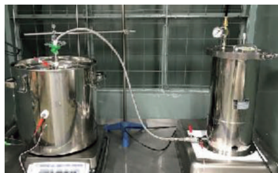
液体の噴霧帯電量の測定 Experimental equipment for measuring of electric charge generated by flow and jet of liquid.
