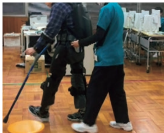
職業性外傷者向け歩行支援機器の介助作業教育 Development of educational tool of walking support equipment for occupational injuries
