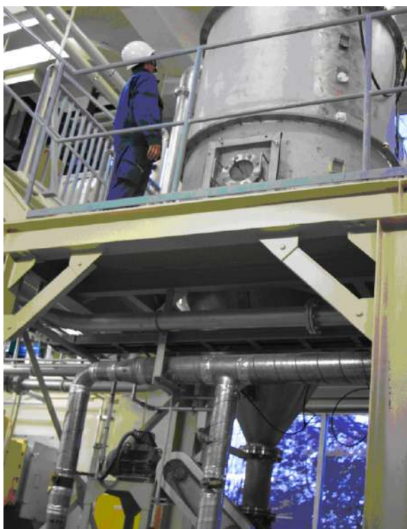
空気輸送粉体の静電気帯電・放電の調査 Pneumatic powder transport facility for investigating electrostatic charges and discharges.
